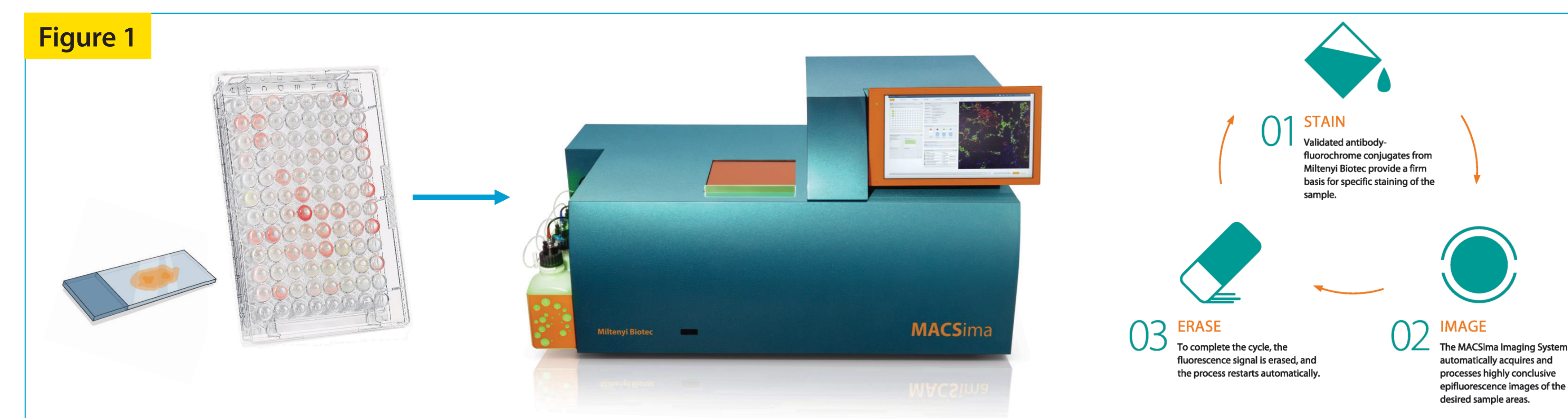
Figure 1. The MICS technology enables the simultaneous analysis of hundreds of markers on a single sample. The cyclic process comprises three main steps that are conducted repeatedly by the MACSima Imaging System in a
