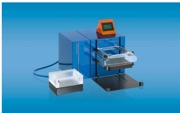
Figure 16: Functional design for the isolation of large sample numbers or volumes with the semi-automated MultiMACS Cell24 Separator Plus.
