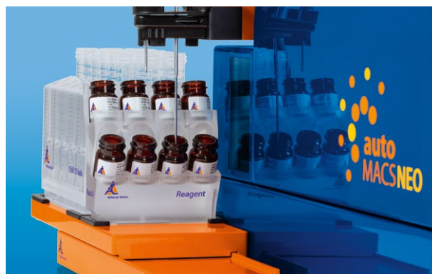
Figure 5: MACS Reagent Rack 8 makes it possible to separate different cell types within multiple samples in one run.
