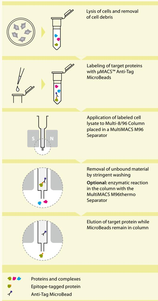
**Figure 9:** Principle of MACS Technology for isolation of epitope-tagged proteins
