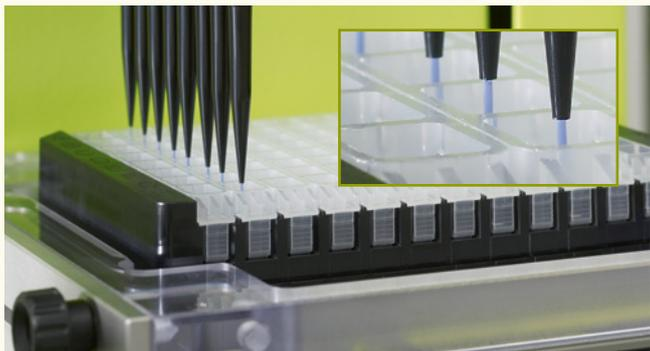
**Figure 8:** Contact-free pipetting for reduced risk of cross-contamination
