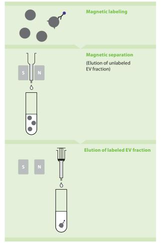
**Figure 1:** Principle of magnetic isolation of EVs using an Exosome Isolation Kit.
