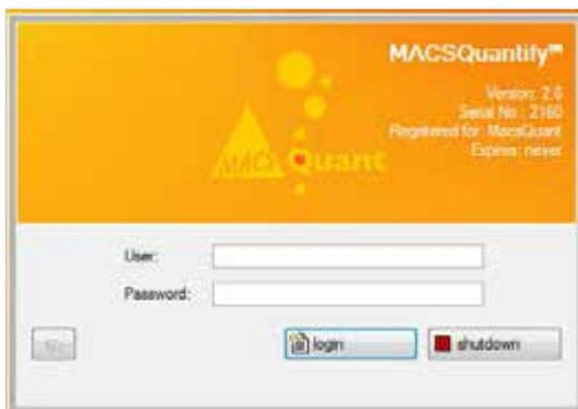
**Note:** After login, the instrument is in data analysis mode. Data acquisition is not yet possible. Prime the instrument before proceeding.
