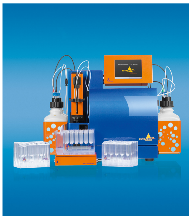
Figure 1: autoMACS ® Pro Separator. Cells of interest are labeled with superparamagnetic nano-sized beads and then passed through a MACS ® Column. When a magnetic field is applied the labeled cells are retained within the column, allowing the unlabeled fraction to be eluted. Once the negative fraction has been eluted, the magnetic field is removed, allowing the labeled cells to be collected in the positive fraction tube.
