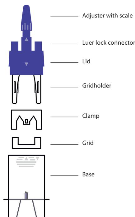
**Figure 1:** Basic illustration of gentleMACS Perfuser components
