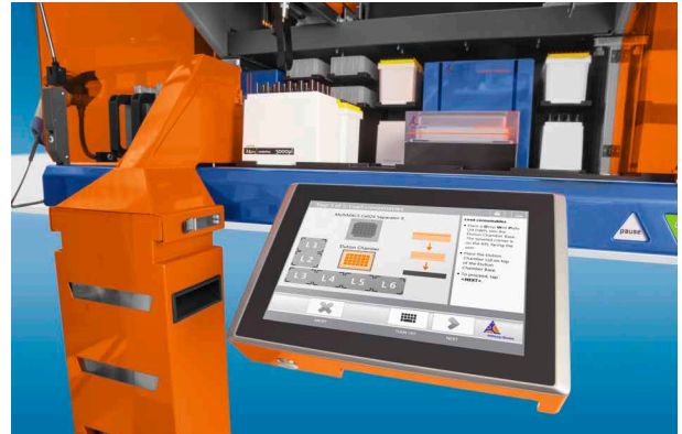
Figure 9: The intuitive user interface guides the user through the loading steps.
