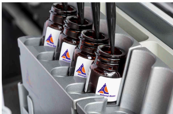
Figure 6: Samples are labeled and incubated on the deck, allowing full walk-away automation.
