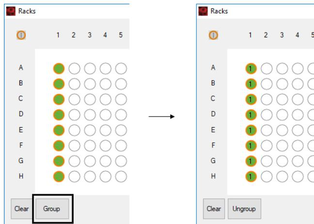
**Figure 2.7:** Select well positions for the samples of one serial dilution and use the **Group** button. Grouped well positions of each serial dilution of the MACSplex Cytokine Standard will be assigned the same group number (example given for a kit with 8 standard positions allowed).
