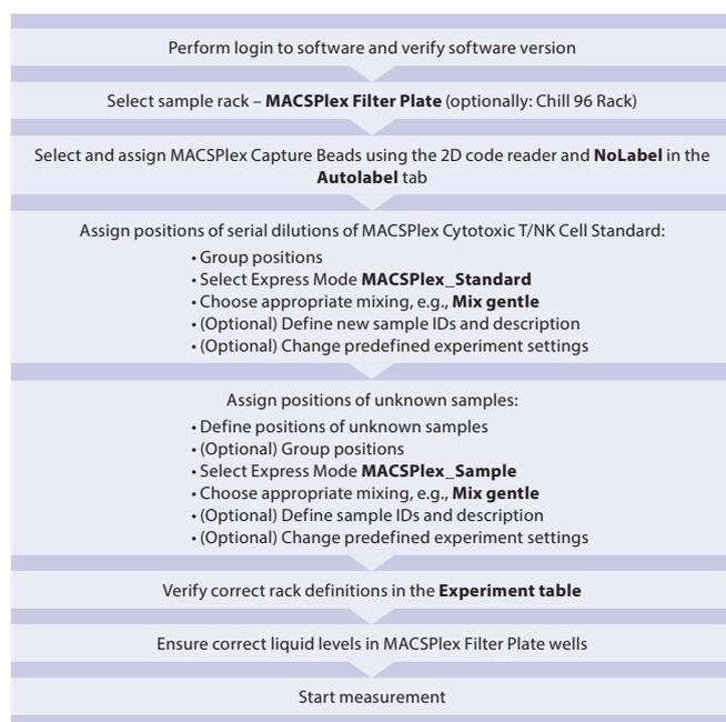
**Figure 2.1:** Overview of data acquisition with a manually defined experiment.
