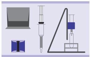
Attach MidiMACS Separator or QuadroMACS Separator to the MultiStand and place Whole Blood Column in the separator. Place a collection tube under the Whole Blood Column.
